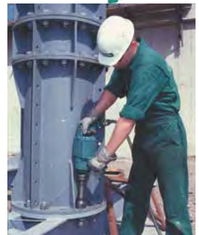
6 1515 0010 3/4" Hydraulic Impact Wrench 1220 ft.-lbs. torque
