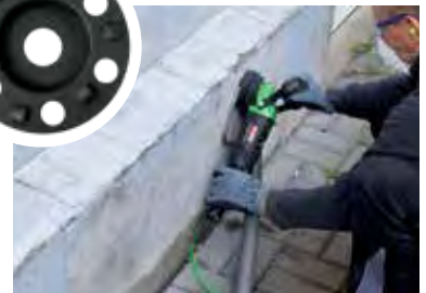
PCD milling disc for concrete surfaces (P/N 37125000)
