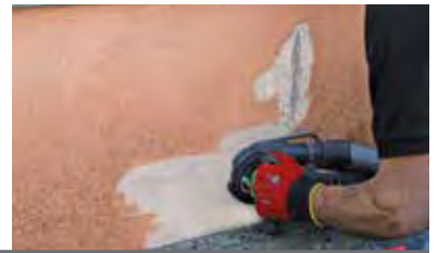
PCD milling disc for concrete surfaces (P/N 37125000)
